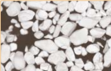
Synthetic Rutile produced by Austpac from the Orissa deposit – grade is 97.5 % TiO 2
