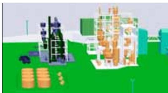
Schematic diagram of a 30,000 tpa ERMS plant (right) and its companion EARS plant
