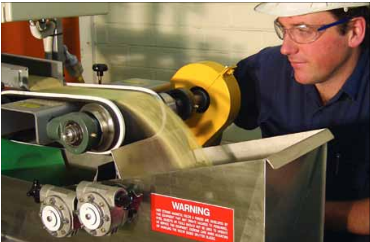
John Winter operating the Rare Earth magnetic separator
