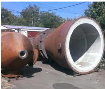
**Refractory-lined fluid bed vessels for gasification and metallisation**
