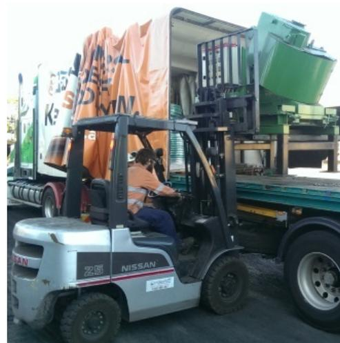
**Unloading the bulk dry sample mixer that will blend the BlueScope iron oxide dusts prior to processing**
