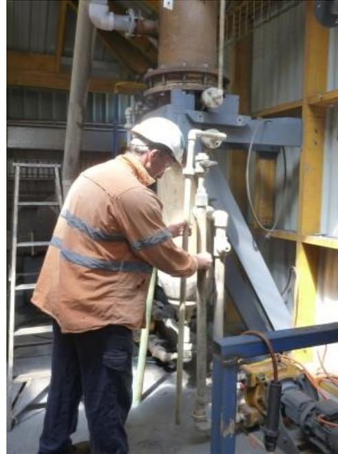
**Adjusting the pipework for the venturi-scrubber (background) to capture and sample roaster gases**
