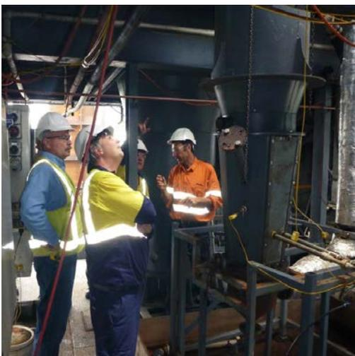
**BlueScope engineers examining the fluid bed evaporator that will process iron oxide dusts**
