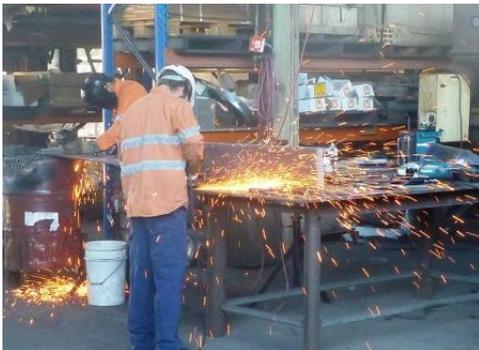
Fabricating steel beams for the North Tower
