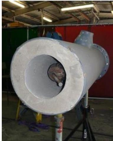
**The batch fluid bed roaster shell ready for installation. This will be used for pyrohydrolysis and metallisation**
