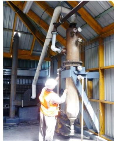
**The venturi-scrubber to recover HCl acid from the batch roaster exit gas streams**
