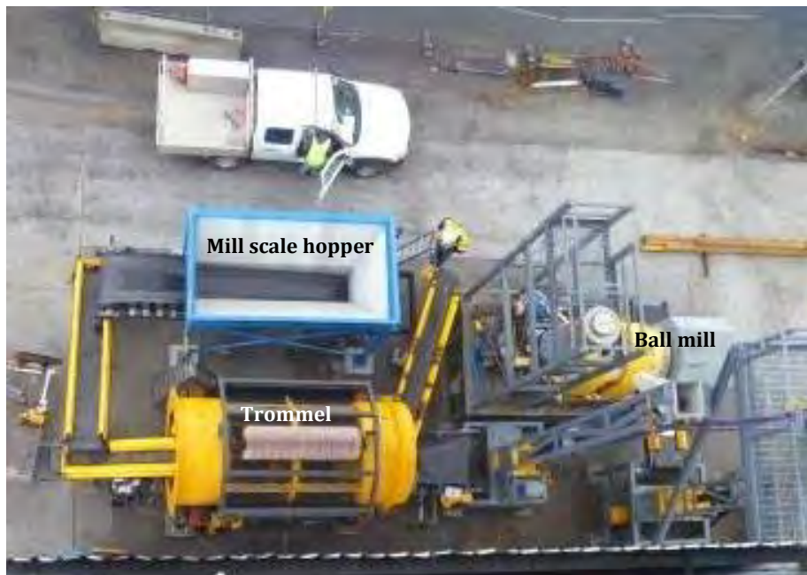
Birds-eye view of the mill scale handling section of the Plant. Raw mill scale will be conveyed from the hopper to the trommel screen, then via an Olds elevator to the ball mill, preparatory to being elevated into the evaporation section in the Plant
