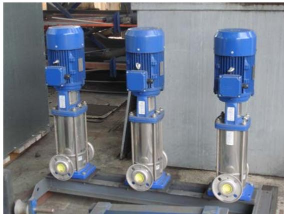
**Process and cooling water pumps awaiting installation**
