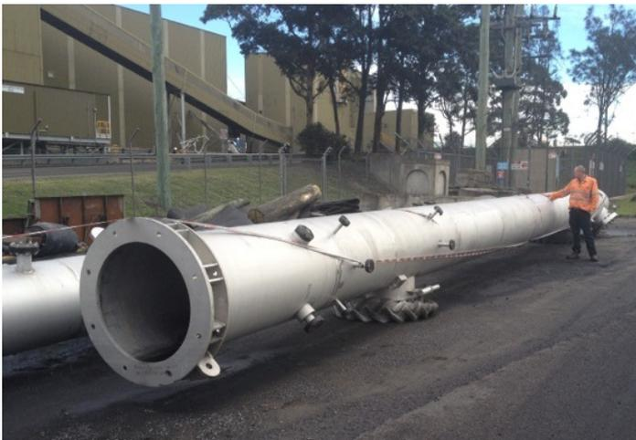
**Absorption columns for CO<sub>2</sub> removal**
