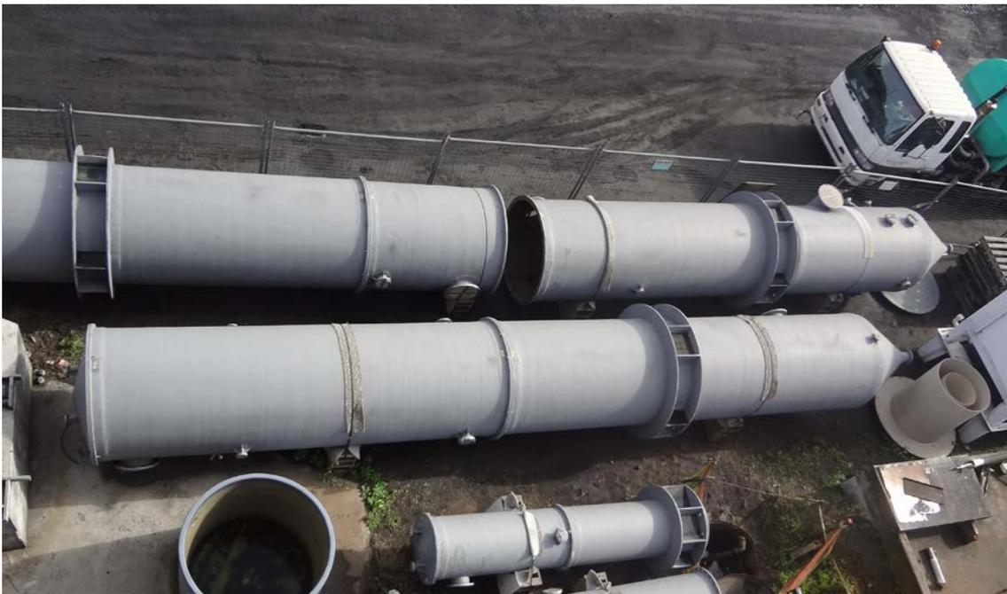
HCl absorption columns for EARS acid regeneration awaiting assembly
