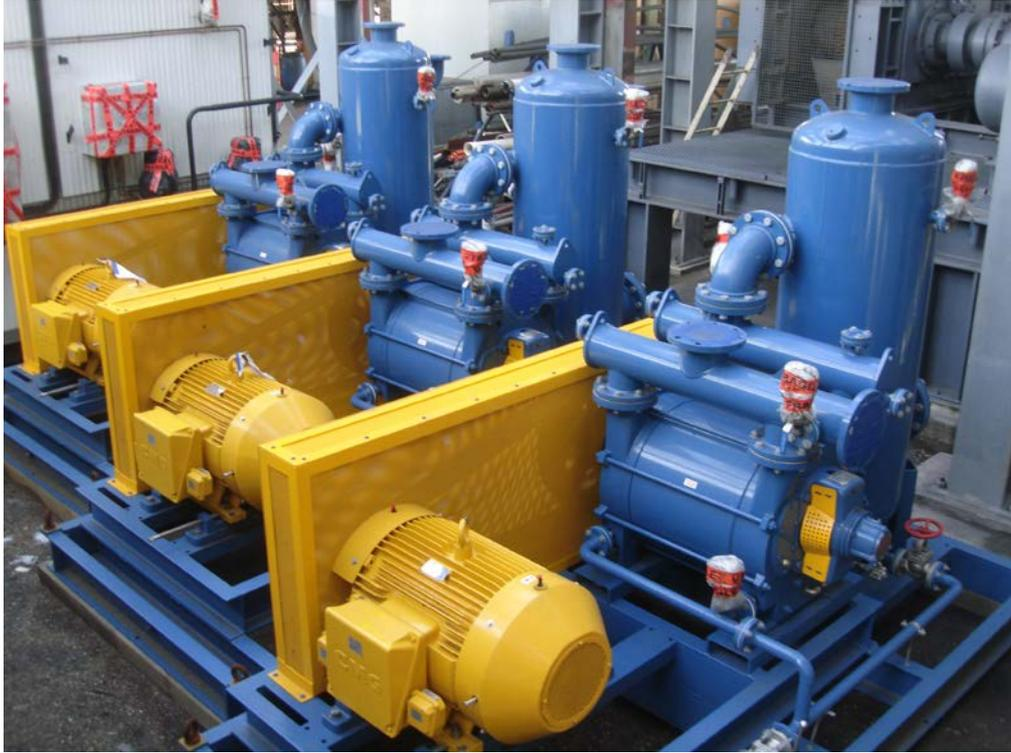
**Liquid ring compressors for gas handling**
