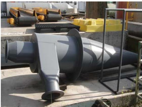
**Cyclone for removal of solids from fluid bed off-gas (mill scale conveyors in background)**
