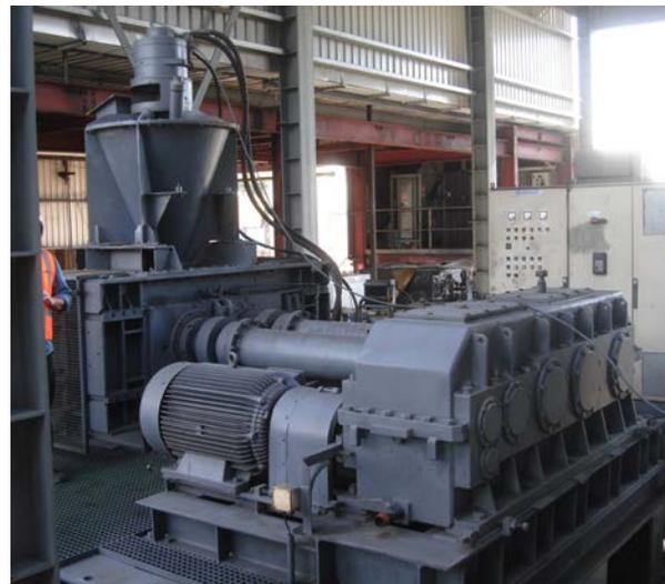
Installed and commissioned briquetter
