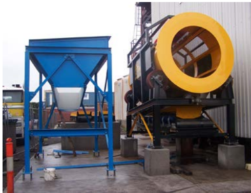
Mill scale feed hopper and rotary screen
