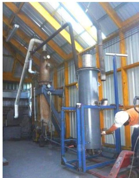
**The batch fluid bed roaster for pyrohydrolysis and iron reduction (foreground) connected to the venturi-scrubber for acid and dust collection**
