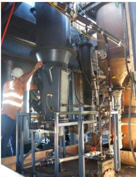
**The fluid bed evaporator being prepared for operation**
