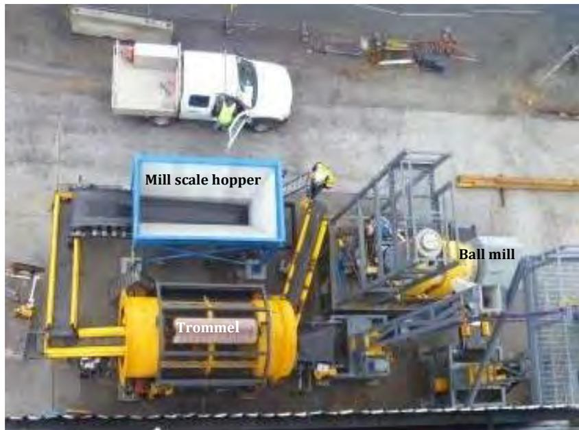
Birds-eye view of the mill scale section of the Plant. Raw mill scale will be conveyed from the hopper to the trommel screen, then via an Olds elevator to the ball mill for homogenisation before being elevated into the Plant
