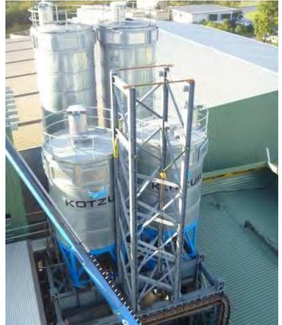
**The completed lower section of the tower. The two silos in the foreground will store iron chips (right) and char (left)**
