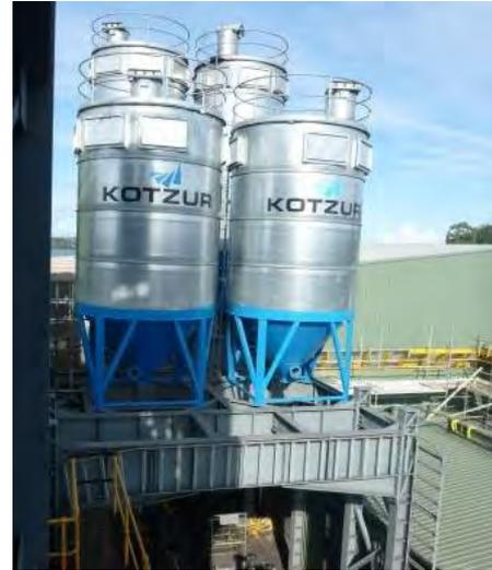
The product and storage silos. The silos in the foreground will hold the two solid products; reduced iron chips (left) and char (carbon) to the right
