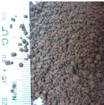
**Iron oxide/iron chloride pellets from evaporation stage**
