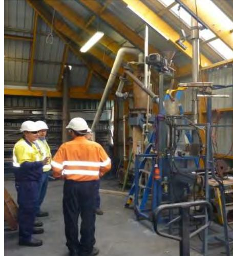
**John Winter explaining the operation of the pilot scale fluid bed roaster to BlueScope engineers**
