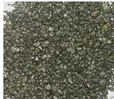
**Iron metal pellets from metallisation stage**
