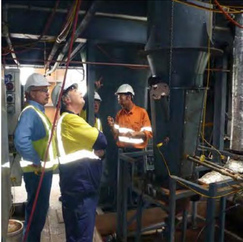
**BlueScope engineers examining the fluid bed evaporator used to process iron oxide dusts**
