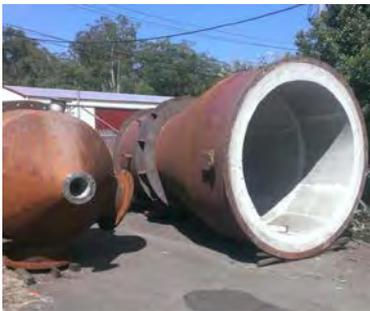
**The gasification and metallisation fluid beds awaiting assembly**
