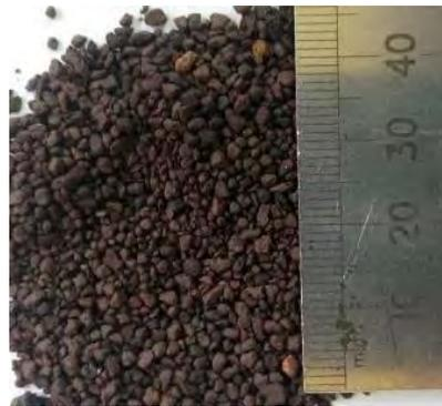
**Iron oxide pellets from pyrohydrolysis stage**
