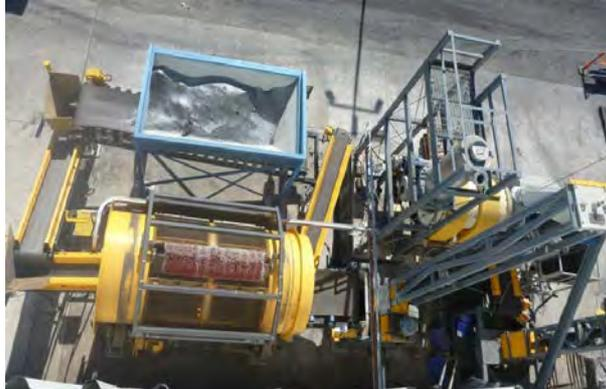
**Mill scale preparation section in operation**
