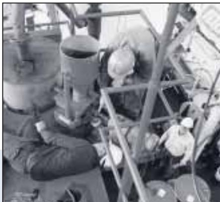
Calibration of ilmenite feed to pre-heat reactor
