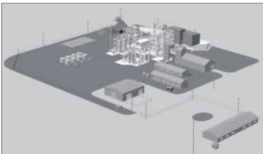
*General layout of proposed AusRutile 10,000 tpa synthetic rutile plant*
