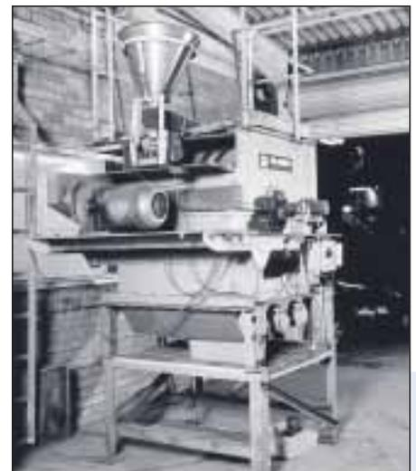
Multi-pole agitated drum magnet at the pilot plant
